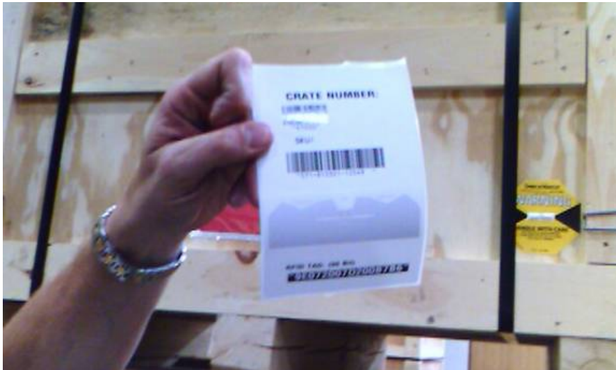
Figure 5 - Passive RFID Label for Tracking Crates of High Value Product
